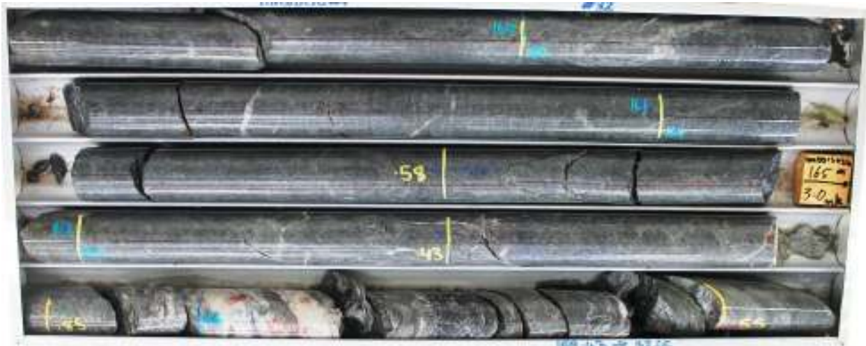
Figure 5. The CMV in AMDD15024 was thin, but contained significant visible gold
